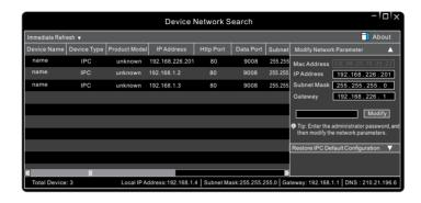
③ Modify the IP address. The default IP address of this camera is 192.168.226.201. Click the information of the camera listed in the above table to show the network information on the right hand. Modify the IP address and gateway of the camera and make sure its network address is in the same local network segment as that of the computer. Please modify the IP address of your device according to the practical situation.
