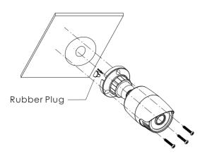
④ Bracket adjustment. Before adjustment, preview the image of the camera on a monitor and then loosen the fixed ring to adjust the view angle of the camera. Tighten the fixed ring after the adjustment.
